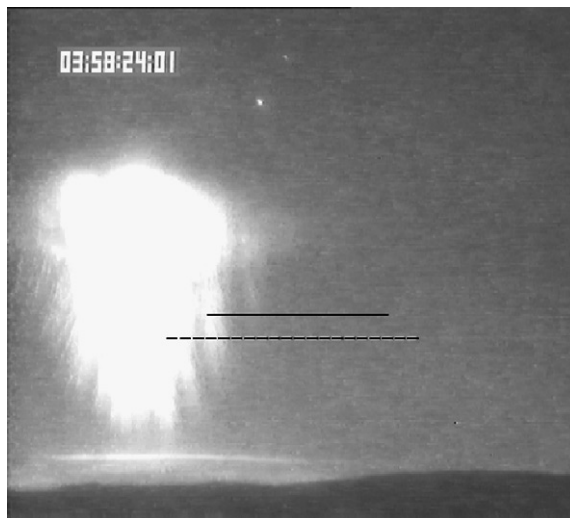
Fig. 1. Image of sprite observed at 03:58 UT on 24 July 1996. Also shown are the slits of the two spectrographs overlaid on the sprite image. The lower, dashed, horizontal line is the projection of the high-resolution ( 70 \text{ \AA} ) spectrograph at 53 km. The upper, solid horizontal line shows the projection of the low-resolution ( \sim 110 \text{ \AA} ) spectrograph at 57 km.
