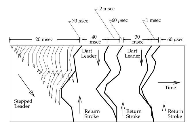
A negative cloud to ground (-CG) lightning flash often has multiple strokes. The figure above (after [4]) illustrates the typical timing of the processes of a multi-stroke -CG. A typical stepped leader has velocity  $\sim 10^5$  m/s while dart leaders have velocity  $\sim 10^6$  m/s.
